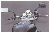
Control lever and switchgear must be protected from excess water during washing by covering with plastic bag!
